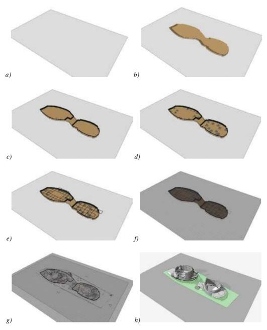
Figure 1: Floating Foundation Workflow. a) Ground Level, b) Excavation of Soil Weight ≥ Building Weight, c) Peripheral Retaining Wall & Thin raft with inverted beam at base, d) Column erected from inverted beam based on column layout, e) Tie
