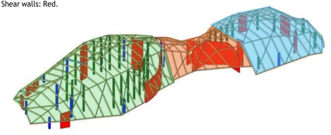
The entire pavilion is split longitudinally into 3 zones as marked above. Each zone has its own structural system for gravity and lateral loads.
