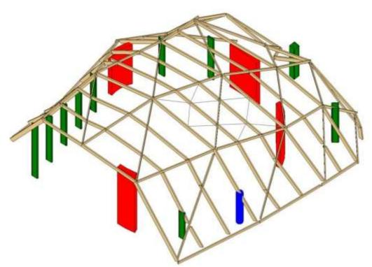
Bracing elements shown only at one location here but will be used over the entire roof.
